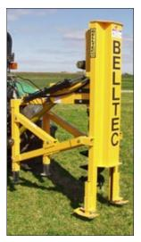
Belltec Industries TM48 Post Hole Digger mounts easily on three-point tractors with over 28 horsepower which have at least two hydraulic remote valves. Our machine's design and performance go way beyond today's tractor mounted post hole diggers.
